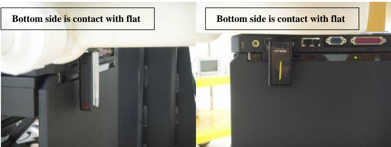
Fig7 : Bottom side of the Notebook is paralleled and contacted with flat phantom.
