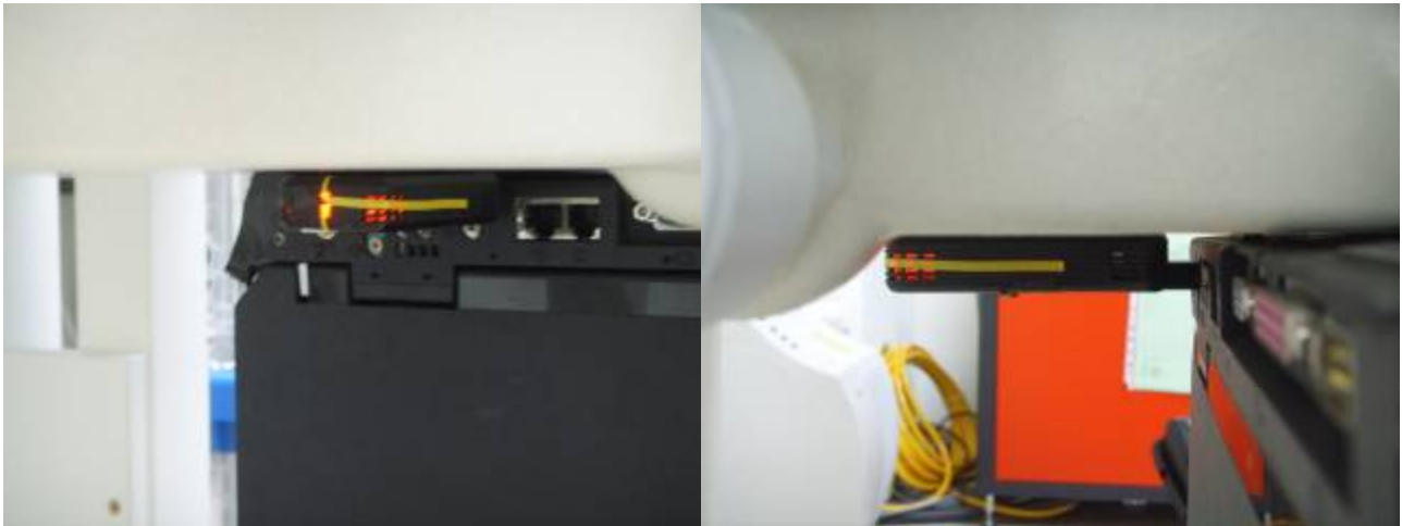
Fig 9: Bottom side of the Notebook is paralleled and contacted with flat Phantom, and front side of the EUT is paralleled with flat phantom.
