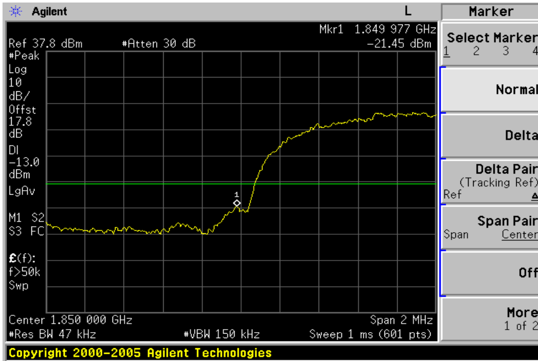
Figure 8-14: Bad edge emission at antenna terminals –WCDMA II Channel Lowest
