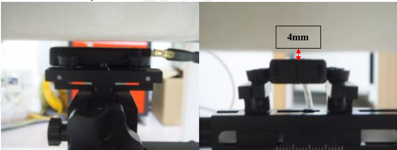
Fig 4 : Rear side of the EUT is paralleled with flat phantom, and spacing between EUT and phantom is 4 mm
