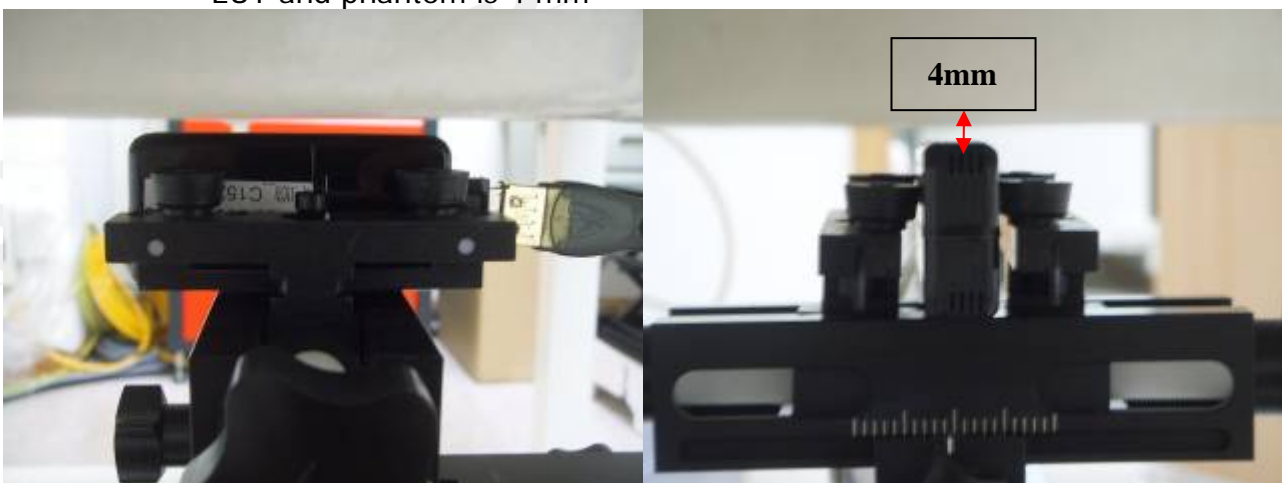
Fig 5 : Right side of the EUT is paralleled with flat phantom, and spacing between EUT and phantom is 4mm
