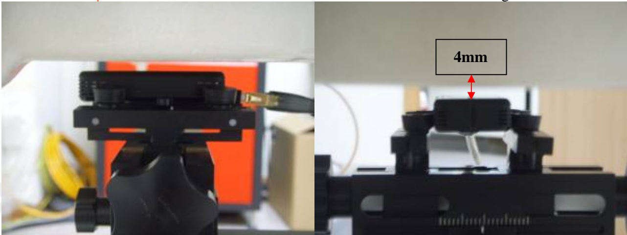
Fig 3 : Front side of the EUT is paralleled with flat phantom, and spacing between EUT and phantom is 4 mm.
