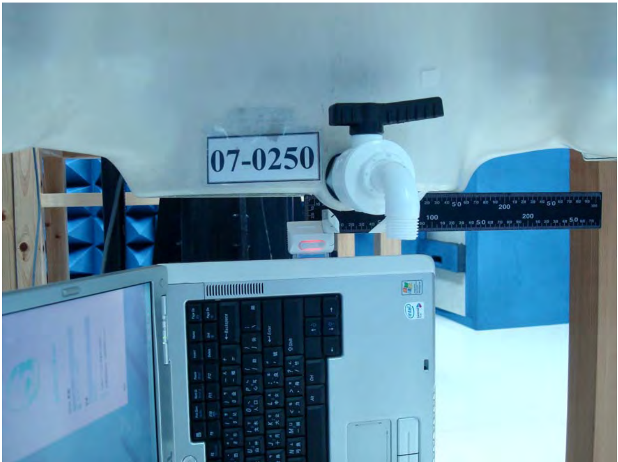
Figure 21. Body SAR Test Setup (Flat Section)_EUT (Antenna Open) Tip to Phantom for NB No.2
