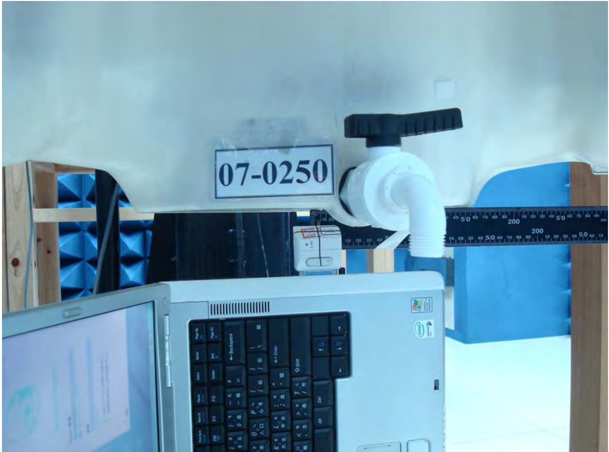
Figure 18. Body SAR Test Setup (Flat Section)_EUT (Antenna Close) Tip to Phantom for NB No.2
