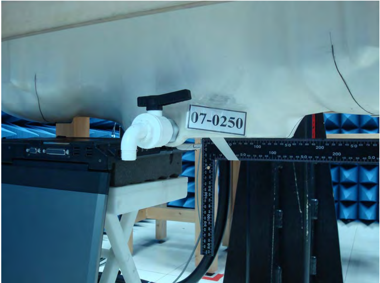
Figure 13. Body SAR Test Setup (Flat Section)_EUT (Antenna Close) Top to Phantom for NB No.3
