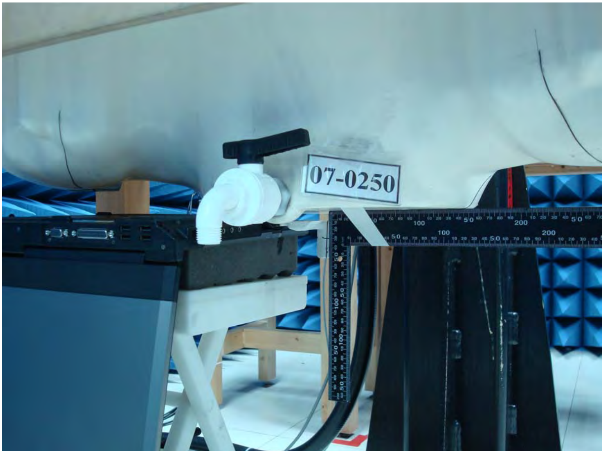
Figure 16. Body SAR Test Setup (Flat Section)_EUT (Antenna Open) Top to Phantom for NB No.3
