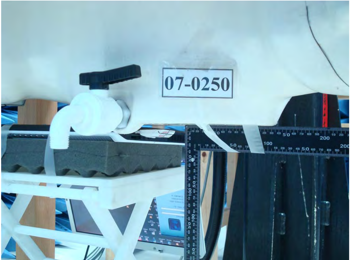
Figure 11. Body SAR Test Setup (Flat Section)_EUT (Antenna Close) Top to Phantom for NB No.1
