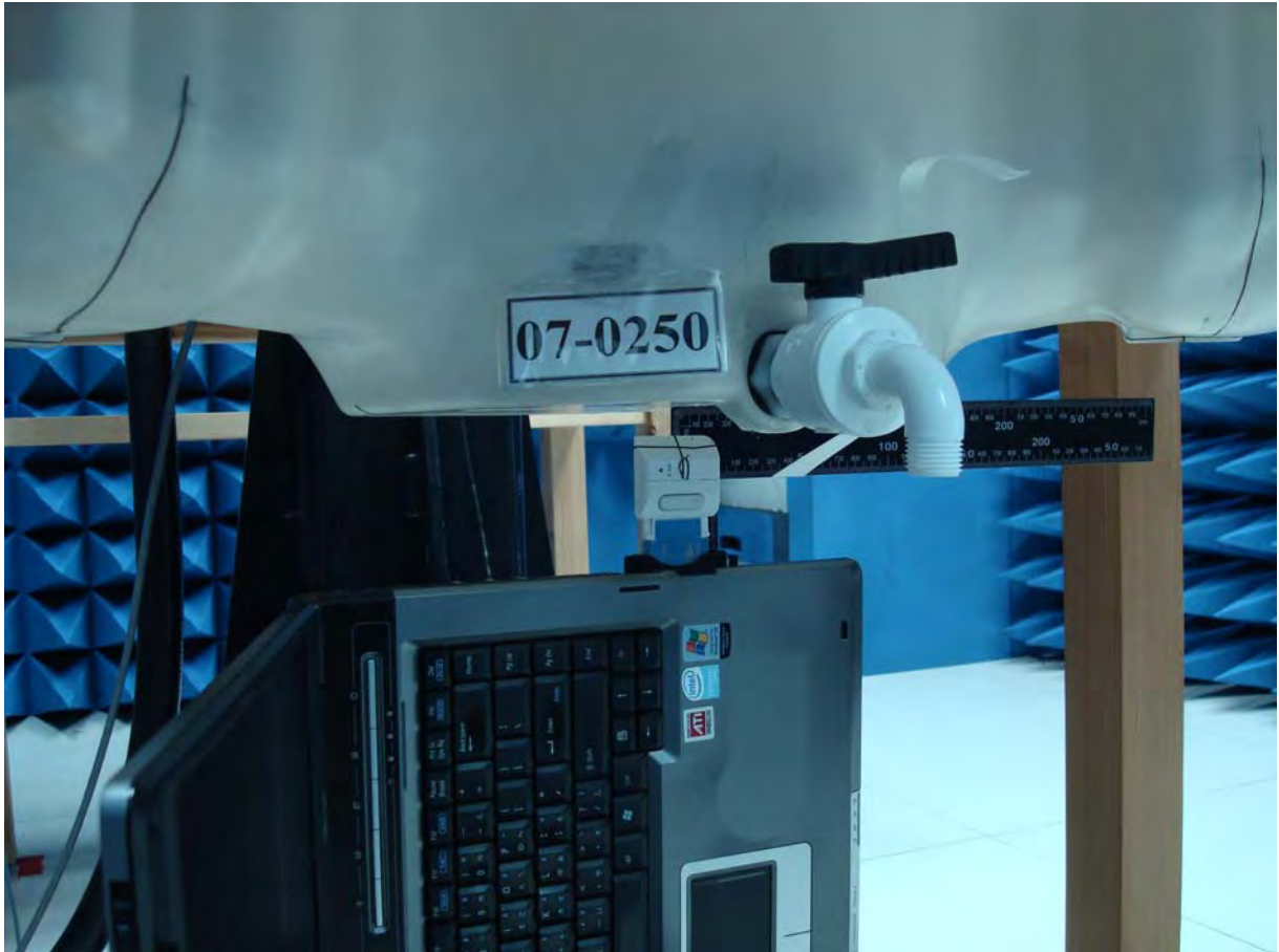
Figure 19. Body SAR Test Setup (Flat Section)_EUT (Antenna Close) Tip to Phantom for NB No.3
