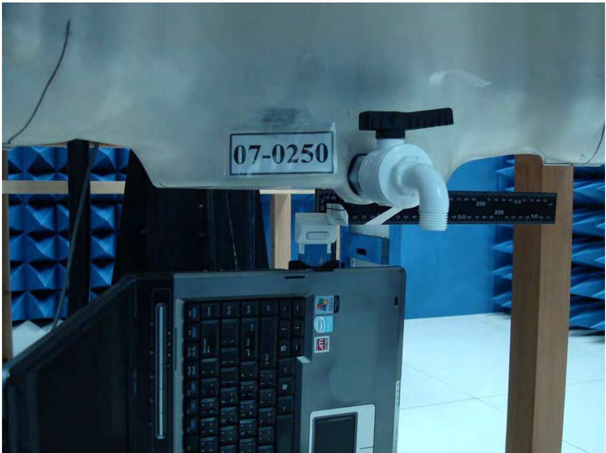
Figure 22. Body SAR Test Setup (Flat Section)_EUT (Antenna Open) Tip to Phantom for NB No.3
