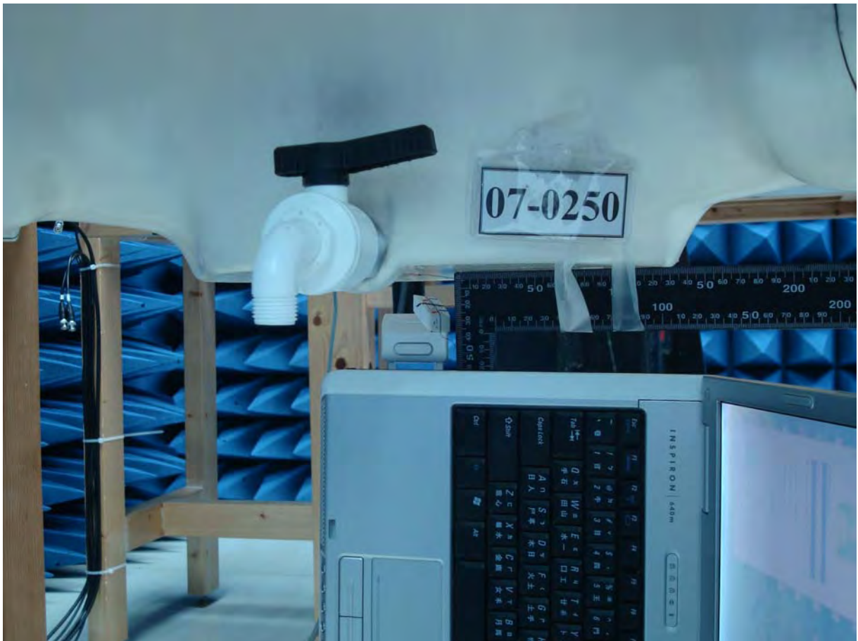
Figure 20.Body SAR Test Setup (Flat Section)_EUT (Antenna Open) Tip to Phantom for NB No.1
