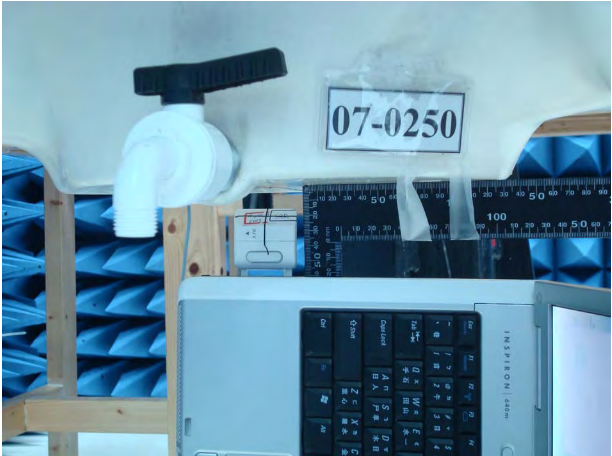
Figure 17. Body SAR Test Setup (Flat Section)_EUT (Antenna Close) Tip to Phantom for NB No.1
