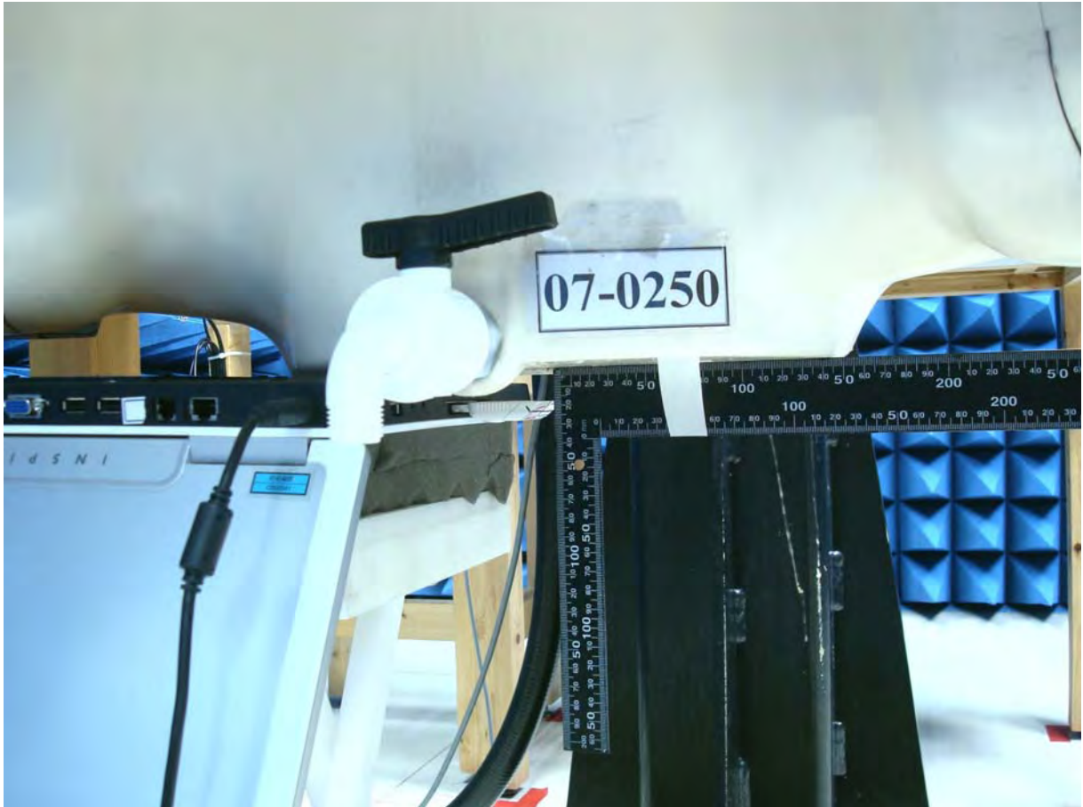
Figure 12. Body SAR Test Setup (Flat Section)_EUT (Antenna Close) Top to Phantom for NB No.2
