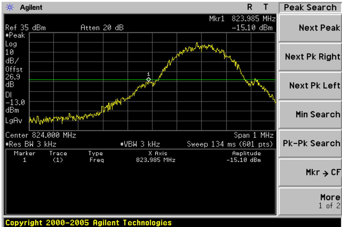
Figure 8-4: Bad edge emission at antenna terminals – GSM Channel Lowest
