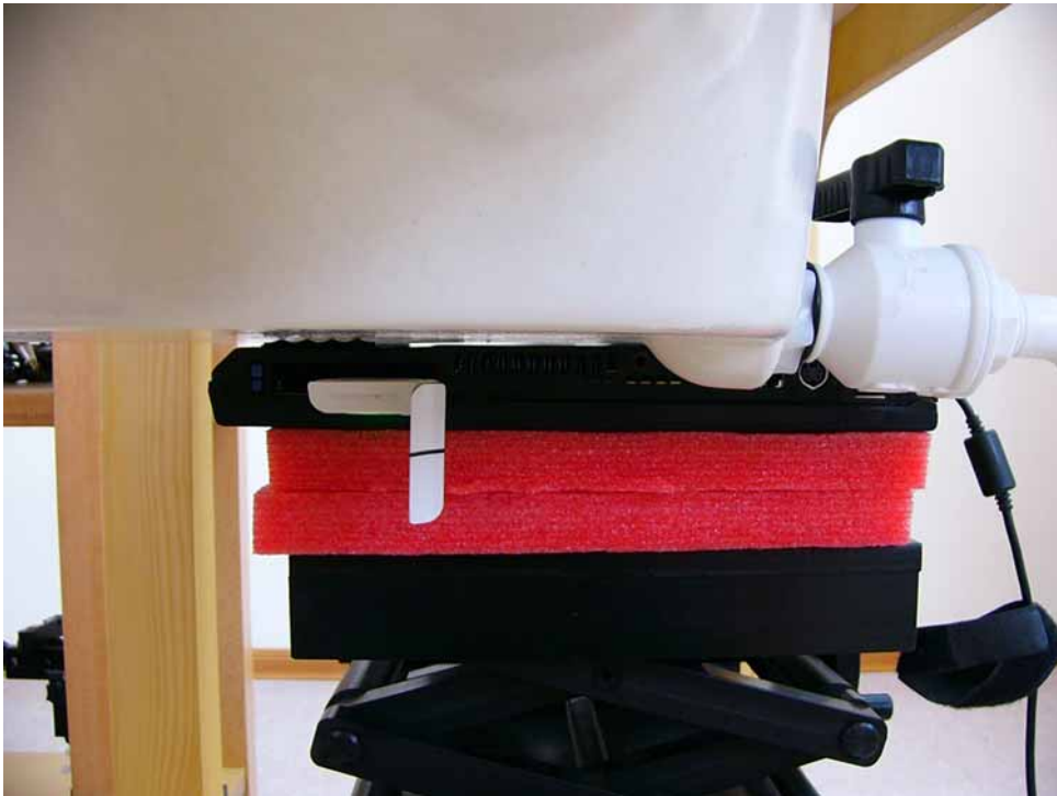
Fig.4.3 Photo of the Bottom face of the notebook is paralleled with flat Phantom, and Antenna of EUT is vertical. (IBM-T43)
