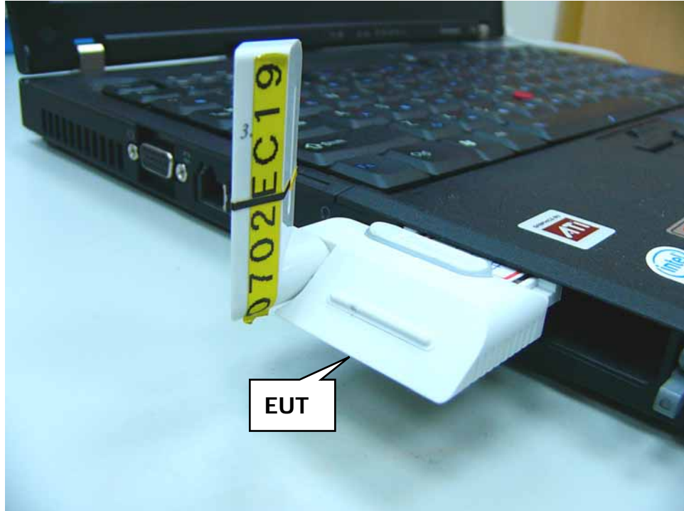
Fig.15 Photograph is express card slot with IBM-T60 (Antenna of EUT is vertical)
