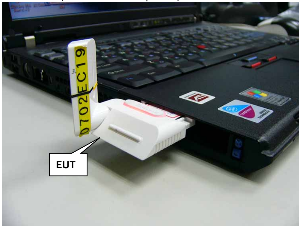
Fig.17 Photograph is express card slot with IBM-T43 (Antenna of EUT is vertical)
