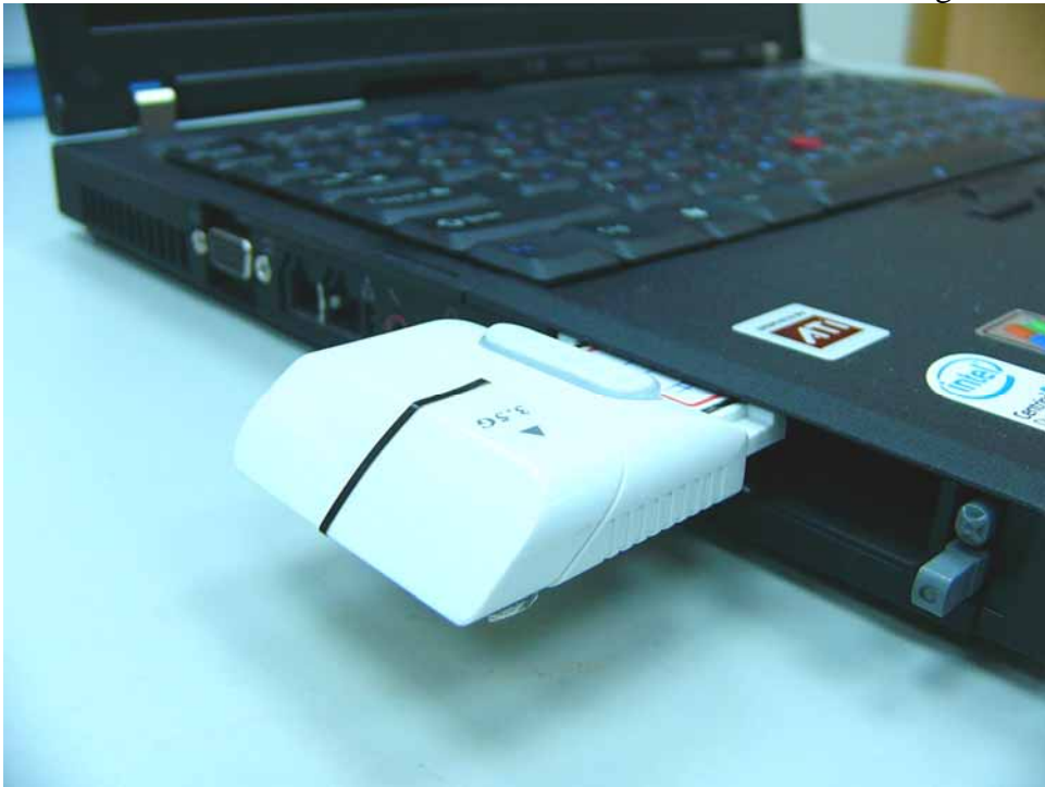
Fig.14 Photograph is express card slot with IBM-T60 (Antenna of EUT is parallel)
