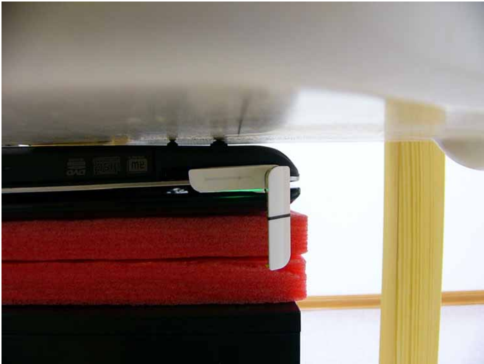
Fig.4.1 Photo of the Bottom face of the notebook is paralleled with flat Phantom, and Antenna of EUT is vertical. (HP-6216)
