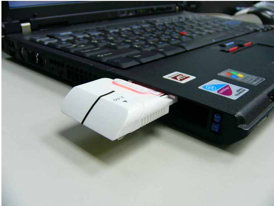
Fig.16 Photograph is express card slot with IBM-T43 (Antenna of EUT is parallel)
