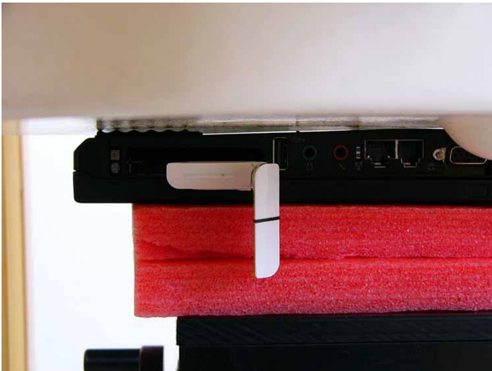
Fig.4.2 Photo of the Bottom face of the notebook is paralleled with flat Phantom, and Antenna of EUT is vertical. (IBM-T60)
