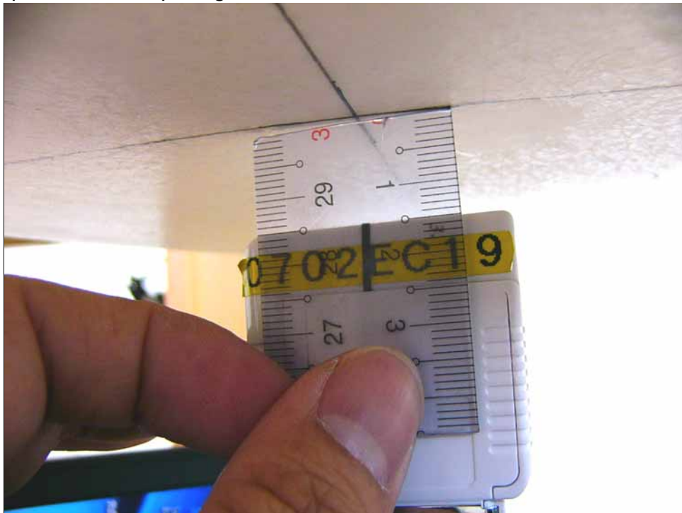
Fig.5.3 Photo is the left side of the Notebook of EUT is vertical with flat phantom and spacing between EUT and Phantom- in contact 15mm.(IBM-T43)
