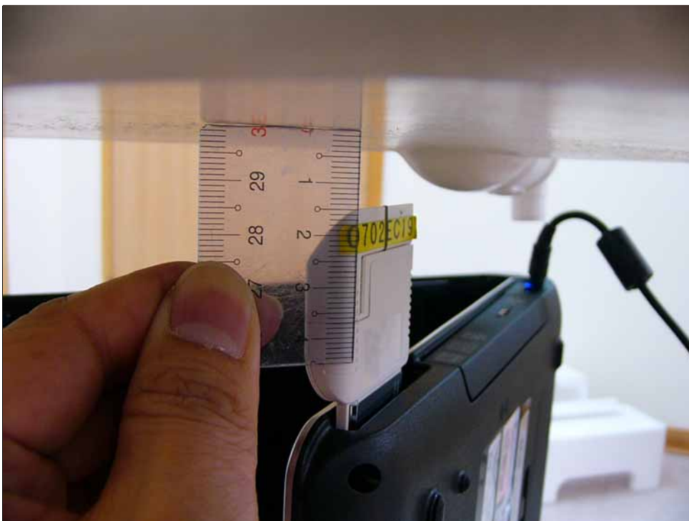
Fig.5.1 Photo is the right side of the Notebook of EUT is vertical with flat phantom and spacing between EUT and Phantom- in contact 15mm.(HP-6216)
