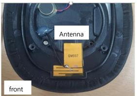
When wearing a headset of the MFB-H7100 model, the distance between the antenna and the human body is 24.6
