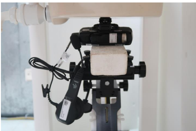
Hip Mount without keypad_Back with headset 1, Test Separation 0 mm
