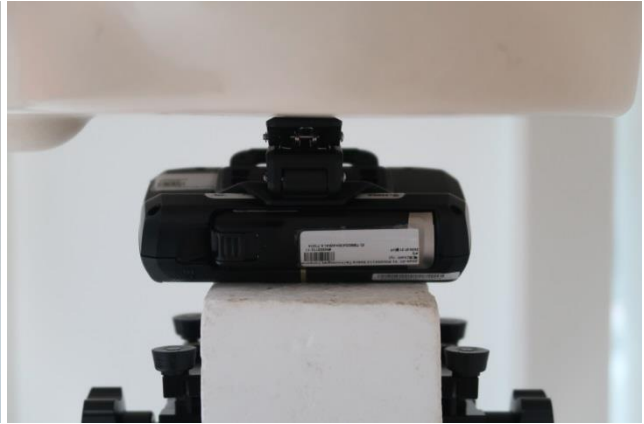
Hip Mount without keypad_Back with battery 1, Test Separation 0 mm
