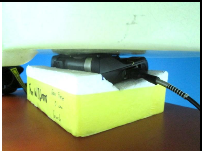
Rear Face of EUT with 0 cm Gap (EUT + Headset 2 + Headset Cable 2 + Wired Scanner 1)
