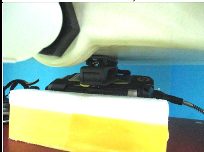
Rear Face of EUT with 0 cm Gap (EUT + Headset 3 + Headset Cable 1 + Wired Scanner 1 + Use Scenario 2)
