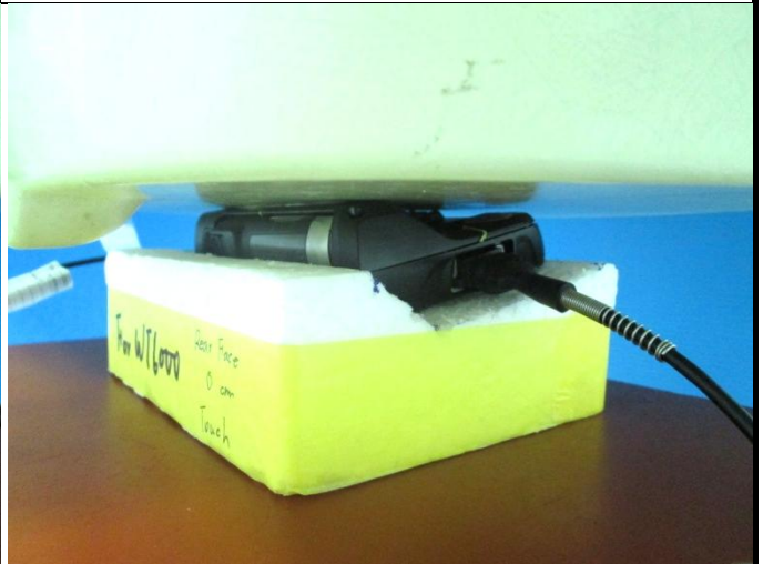
Rear Face of EUT with 0 cm Gap (EUT + Headset 3 + Vibrator Cable 1 + Headset Cable 2)
