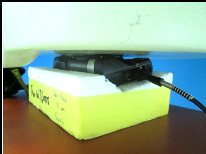
Rear Face of EUT with 0 cm Gap (EUT + Headset 3 + Headset Cable 2 + Wired Scanner 1)
