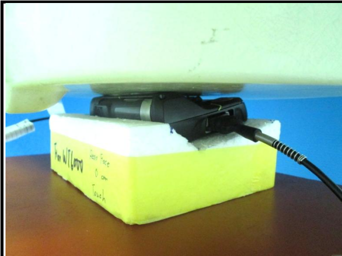
Rear Face of EUT with 0 cm Gap (EUT + Headset 2 + Vibrator Cable 1 + Headset Cable 2)
