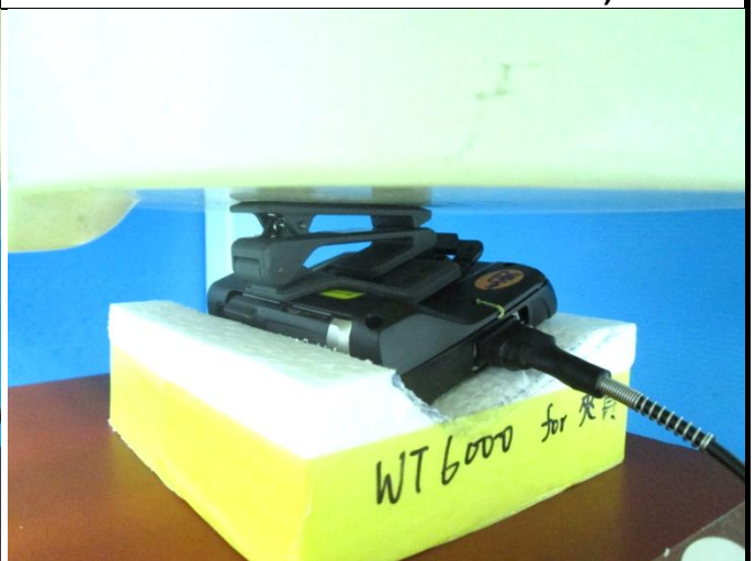
Rear Face of EUT with 0 cm Gap (EUT + Headset 4 + Headset Cable 2 + Use Scenario 2)
