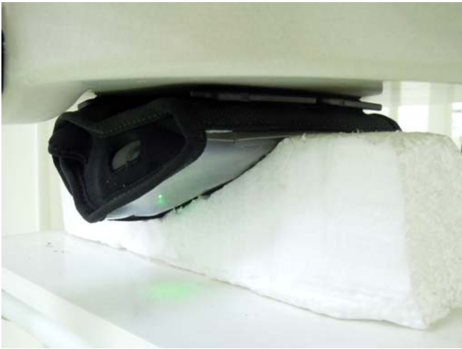
Rear Face of EUT with 0 mm Gap (EUT + Battery 1 + Holster 1)
