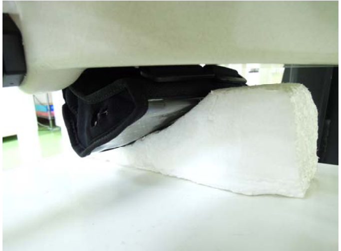
Rear Face of EUT with 0 mm Gap (EUT + Battery 2 + Holster 1)
