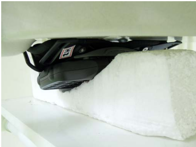
Rear Face of EUT with 0 mm Gap (EUT + Battery 1 + Holster 2)
