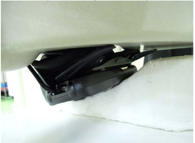
Rear Face of EUT with 0 mm Gap (EUT + Battery 2 + Holster 2)
