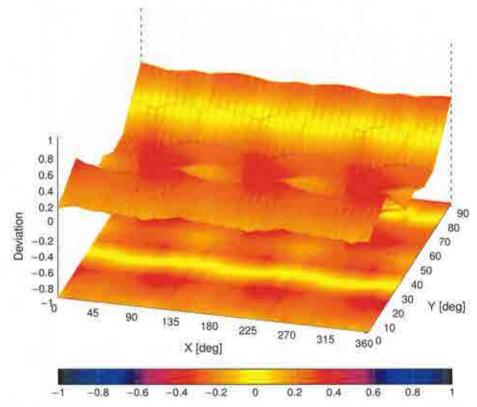
Probe isotropy for  $E_{tot}$ : probe rotated  $\psi=0^\circ$  to  $360^\circ$ , tilted from field propagation direction  $\vec{k}$  Parallel to the field propagation ( $\psi=0^\circ-90^\circ$ ) at 30 GHz: deviation within  $\pm 0.32$  dB Parallel to the field propagation ( $\psi=0^\circ-90^\circ$ ) at 60 GHz: deviation within  $\pm 0.44$  dB
