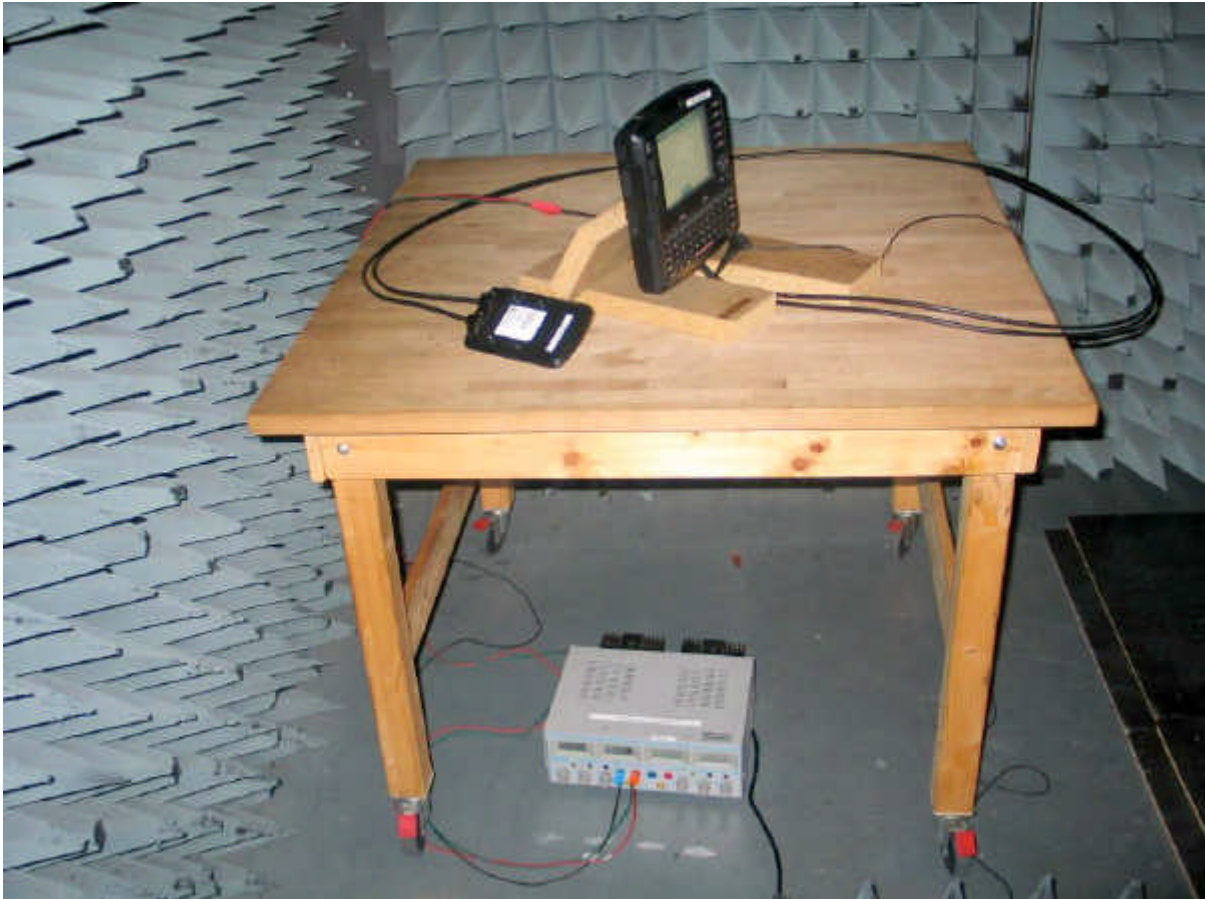
Photo 1: Test setup for radiated measurements (up to 30 MHz)
