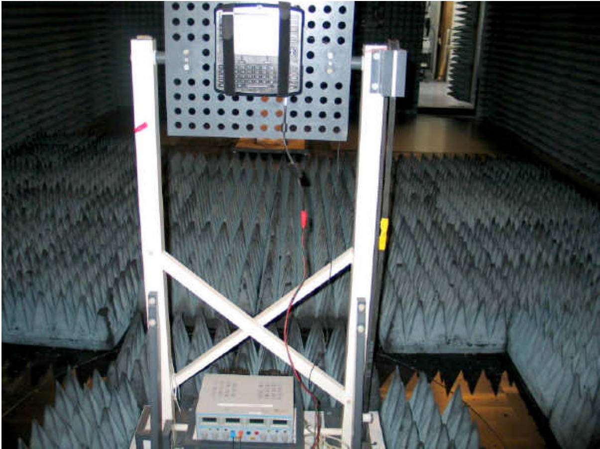
Photo 3: Test setup for radiated measurements (above 1 GHz)
