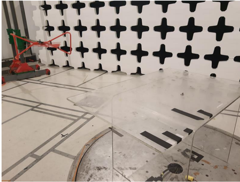
Photograph 1. Radiated Spurious Emissions Test Setup, 30-1000MHz
