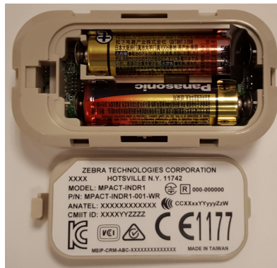
Figure 4-10 Open Battery Enclosure: MPACT-MB2000-01-WR
