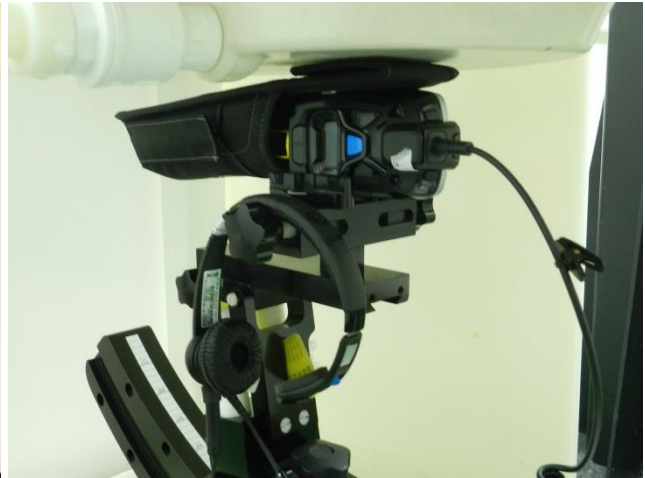
(SE965) Right Side with Holster1 + Headset 2 Test Separation 0 mm
