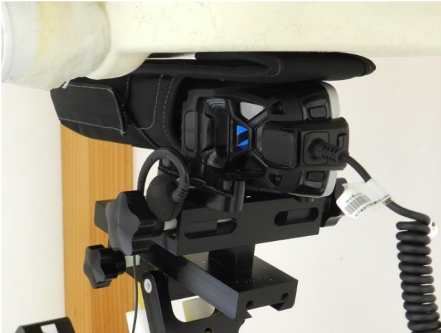
(SE965) Right Side with Holster1 + Headset 1 Test Separation 0 mm
