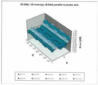
Probe isotropy for  $E_{tot}$ : probe rotated  $\phi=0^\circ$  to 360°, tilted from field propagation direction  $\bar{k}$  Parallel to the field propagation ( $\psi=0^\circ$  - 90°) at 30 GHz: deviation within  $\pm$  0.29 dB Parallel to the field propagation ( $\psi=0^\circ$  - 90°) at 60 GHz: deviation within  $\pm$  0.45 dB
