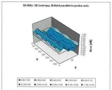
Probe isotropy for E<sub>tot</sub>: probe rotated  $\phi$  = 0° to 360°, tilted from field propagation direction  $\overline{k}$  Parallel to the field propagation ( $\psi$  =0° - 90°) at 30 GHz: deviation within ± 0.42 dB Parallel to the field propagation ( $\psi$  =0° - 90°) at 60 GHz: deviation within ± 0.46 dB
