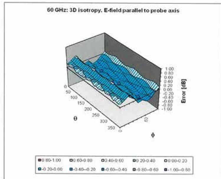
Probe isotropy for  $E_{\text{tot}}$ : probe rotated  $\varphi = 0^\circ$  to  $360^\circ$ , tilted from field propagation direction  $\vec{k}$
