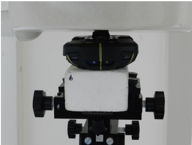
Front with Rigid Holster, Test Separation 0 mm
