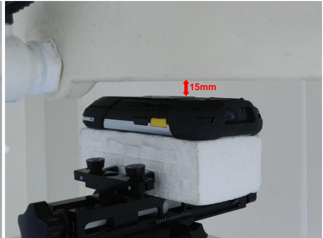
Back , Test Separation 15 mm
