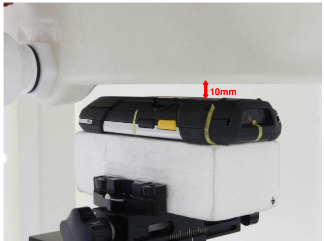
Back, Test Separation 10 mm
