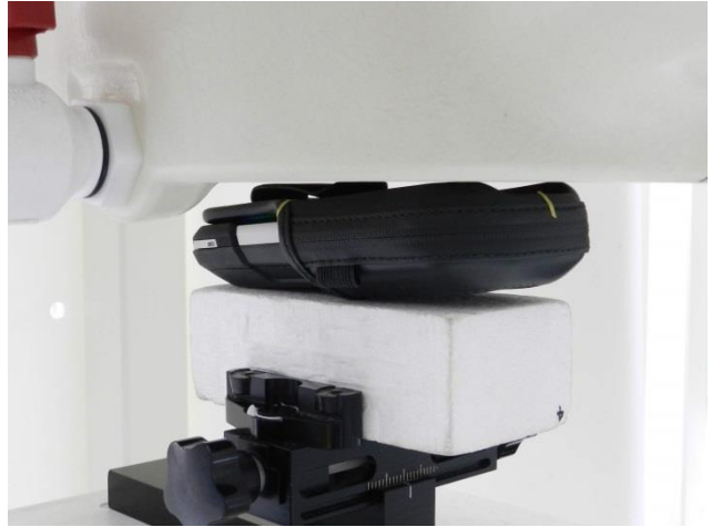
Front with soft holster, Test Separation 0 mm
