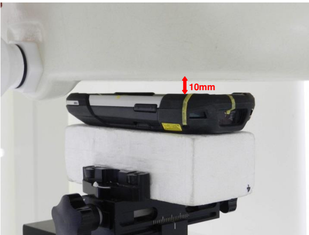
Front, Test Separation 10 mm
