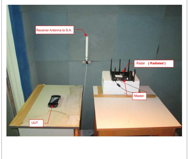
Set UUT as Client without radar detection mode (Radar injected into Master)
