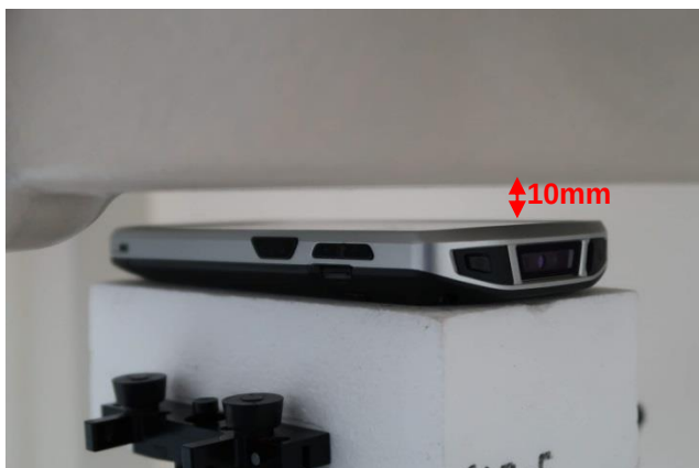
Front, Test Separation 10 mm
