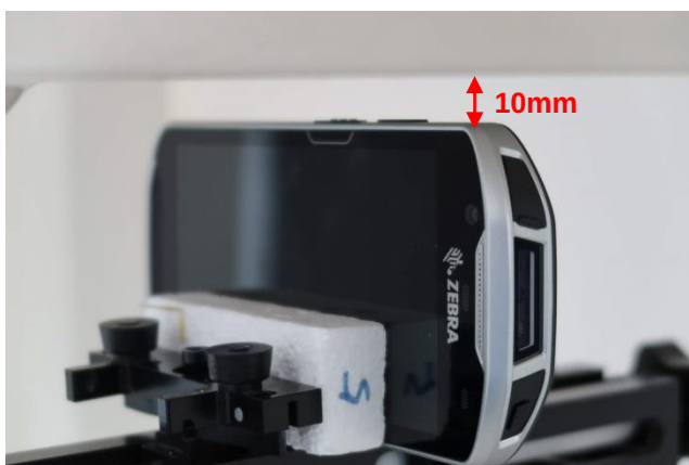
Left Side, Test Separation 10 mm
