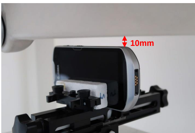
Right Side, Test Separation 10 mm
