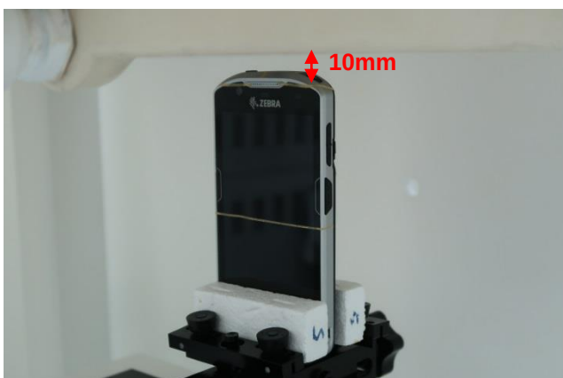
Top Side, Test Separation 10 mm
