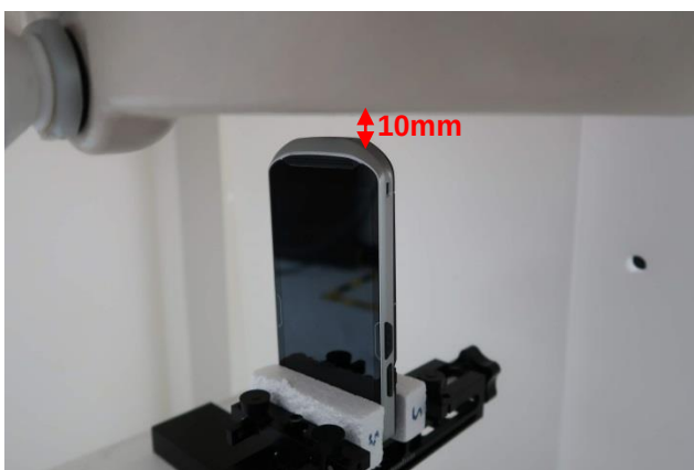
Bottom Side, Test Separation 10 mm
