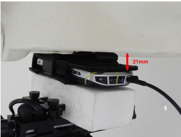
Front with Soft Holster + 2.5mm Earphone, Test Separation 0 mm
