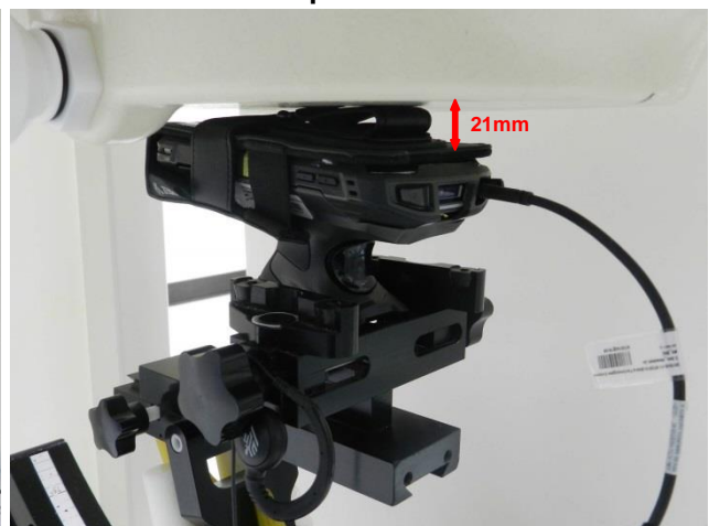
Front with Soft Holster + Exoskeleton + Trigger Handle + 3.5mm Earphone, Test Separation 0 mm
