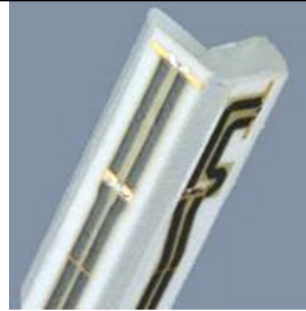
Fig 5.2 Photo of E-field Probe
