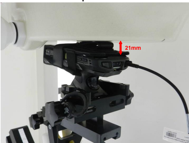
Front with Soft Holster + Exoskeleton + Trigger Handle + 2.5mm Earphone, Test Separation 0 mm
