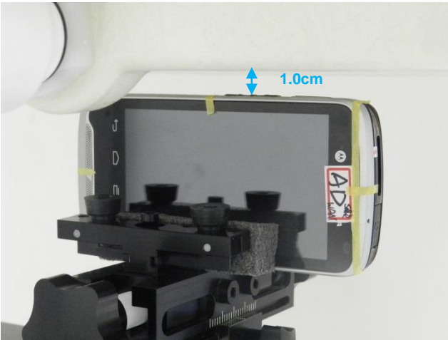
Left Side With Battery 1, Test Separation 1 cm
