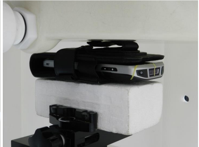
Front with Soft Holster, Test Separation 0 mm
