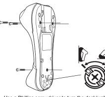
1. Use a Phillips screwdriver to turn the desk/wall mount converter knob to the position shown below. The front latches protract to engage the depressions at the base of the scanner's handle 2. Attach the interface and power cables to the appropriate ports (see
