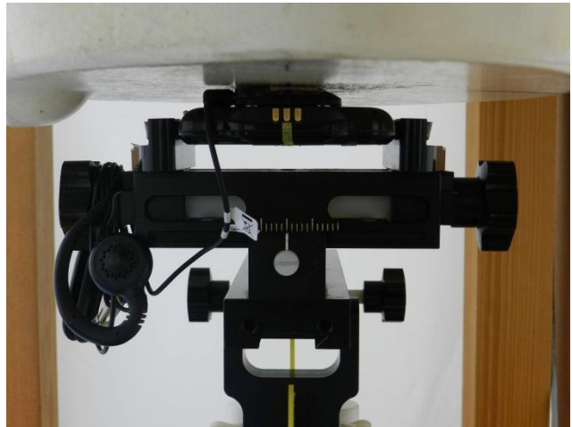
Back of the EUT with Headset nugget with Headset 2 at 0 cm Gap
