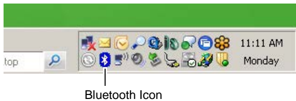
Figure 68 HID - Bluetooth Icon On Computer Desktop Tray - Windows XP SP3 and Bluetooth V2.1
