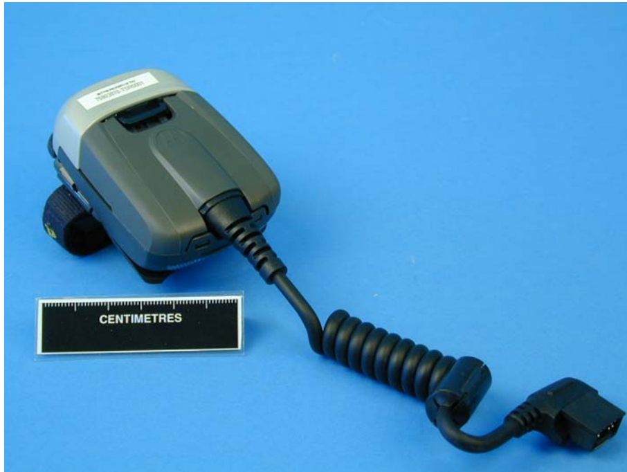
Equipment Under Test with direct cable link
