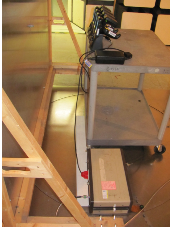
Conducted Emissions Four Slot Charger
