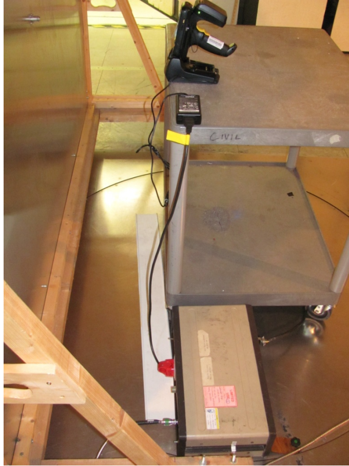
Conducted Emissions Single Slot Charger
