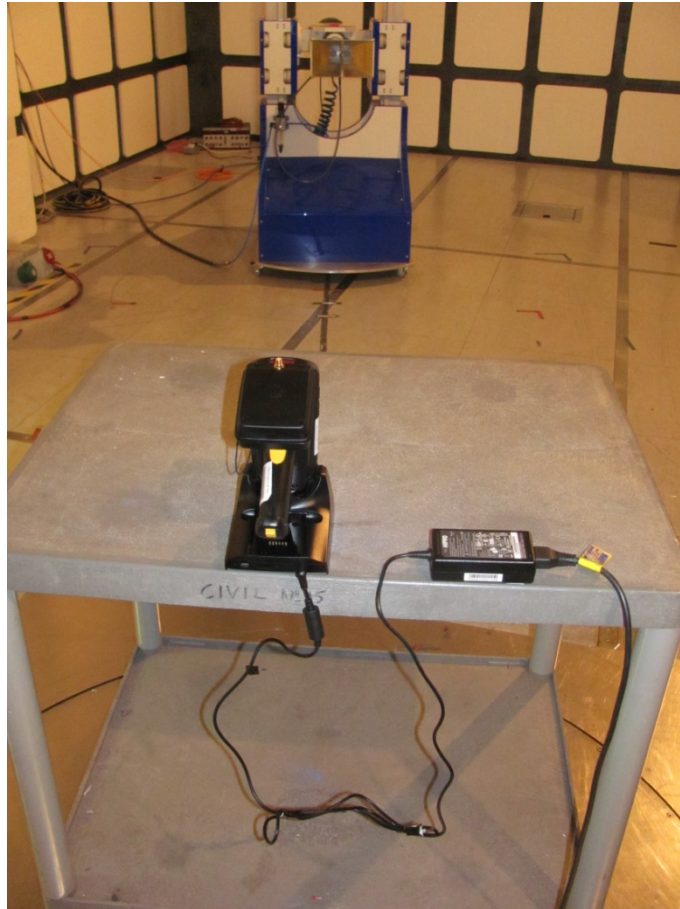
Radiated Emissions 1-25GHz Single Slot Charger
