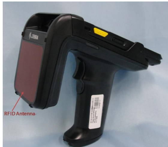
RFID Antenna Location
