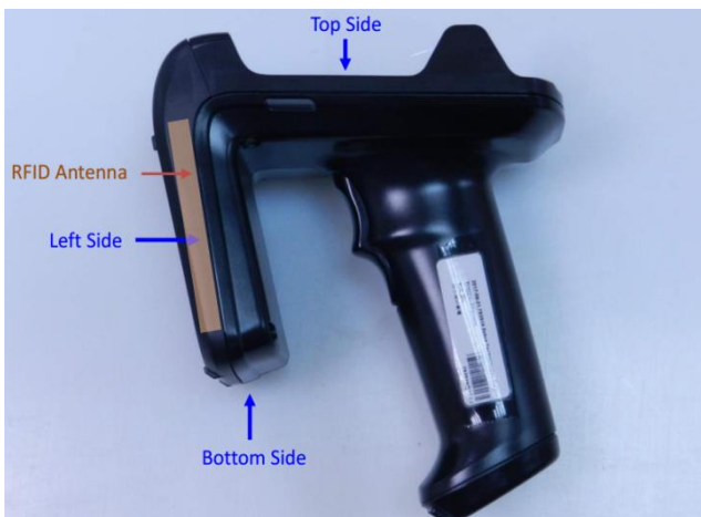
Left Side View (RFID terminal)
