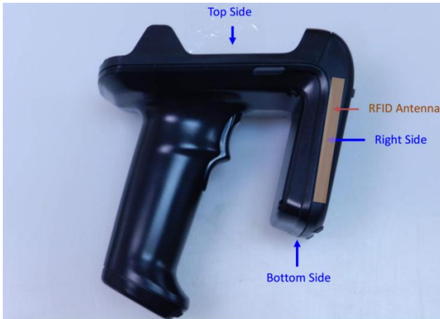
Right Side View (RFID terminal)
