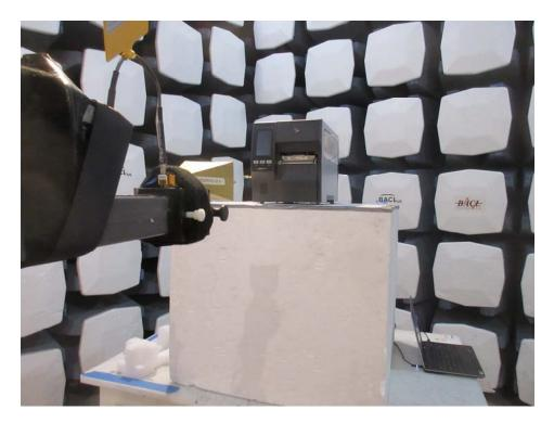
1.6 Radiated Spurious Emissions measured at 1 meter, 18 GHz to 26.5 GHz, Rear View
