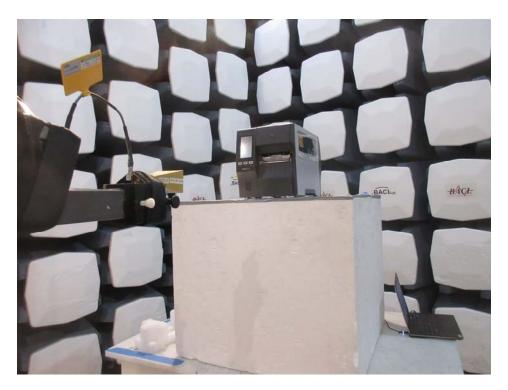
1.8 Radiated Spurious Emissions measured at 1 meter, 26.5 GHz to 40 GHz, Rear View
