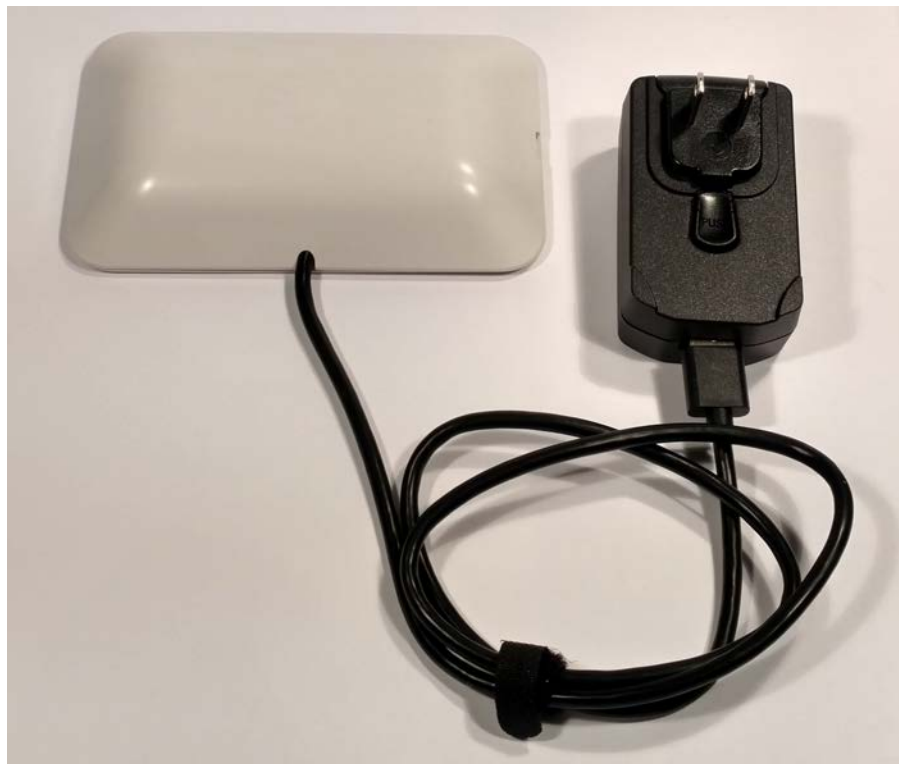
Figure 29 Hub with Power Connected
