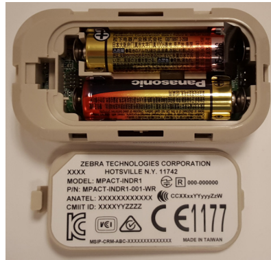
Figure 2-10 Open Battery Enclosure: MPACT-MB2000-01-WR
