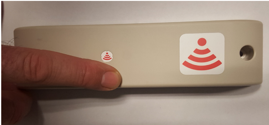
Figure 2-16 Activating Outdoor Style Beacon - MPACT-MB4000-01-WR
