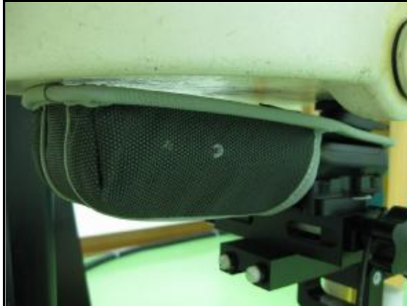
The front of the EUT face to the phantom with 0mm-separation distance.
