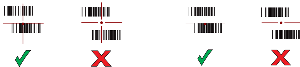
Figure 28 Pick List Mode with Multiple Barcodes in Aiming Pattern: Standard and Extended Range
