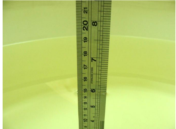
Fig 6.2 Photo of Liquid Height for Body SAR
