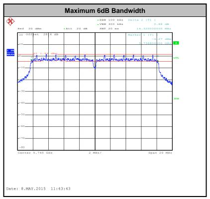
**Note:** The occupied channel bandwidth is maintained within the band of operation for all of the modulations.
