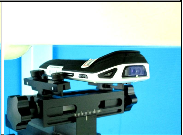
Rear Face of EUT with 1.5 cm Gap
