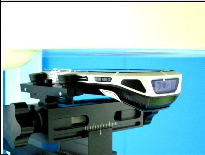
Front Face of EUT with 1.5 cm Gap
