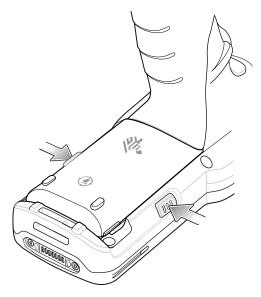
2. Remove the battery from the battery compartment.
