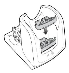
4. Insert the device into the MC32N0 cradle.
