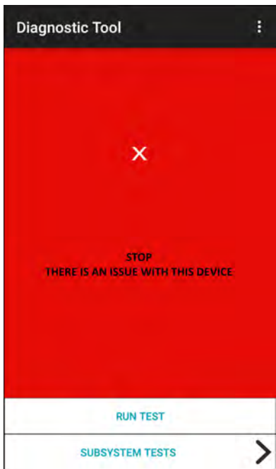
Figure 45 Test Failed Screen
