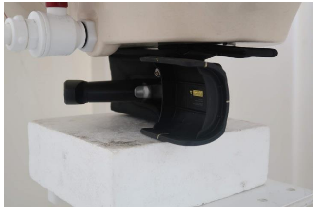
Right Side with holster, Test Separation 0 mm
