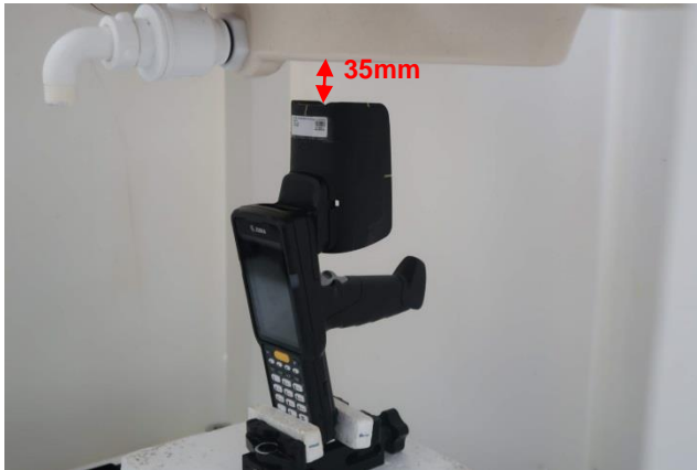
Front, Test Separation 35 mm
