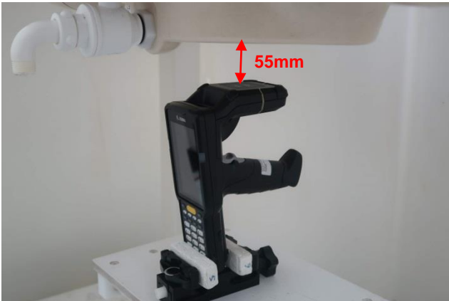
Front, Test Separation 55 mm
