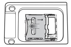
6. Replace the microSD card cover and ensure that it is installed properly.
