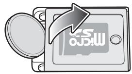
2. Slide the microSD card holder to the Open position.
