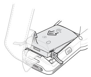
3. Align the battery into the battery compartment.
