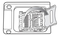
4. Place the microSD card into the contact area with the contacts facing down.
