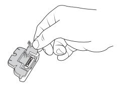
**3.** Insert the adapter into the MC32N0 cradle and adhere it to the bottom of the cradle.
