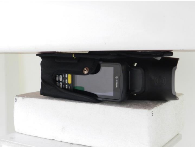
Left Side with holster, Test Separation 0 mm
