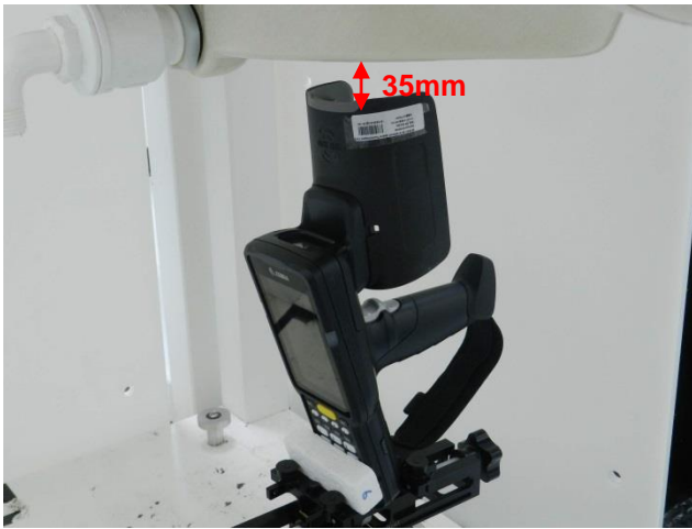
Front, Test Separation 35 mm
