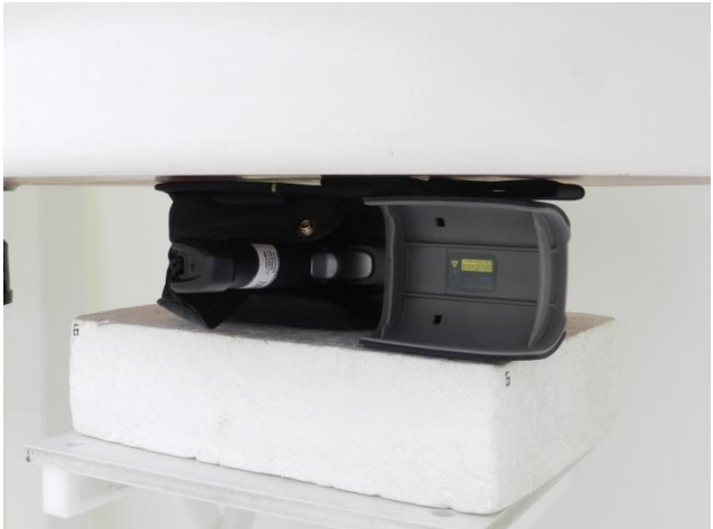
Right Side with holster, Test Separation 0 mm
