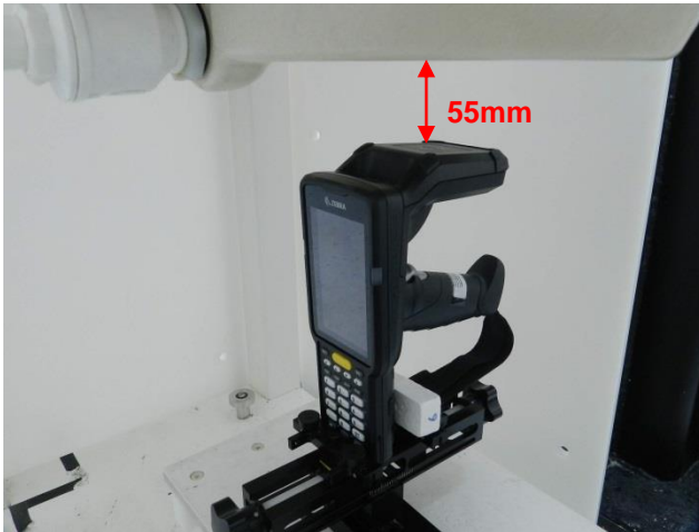
Front, Test Separation 55 mm
