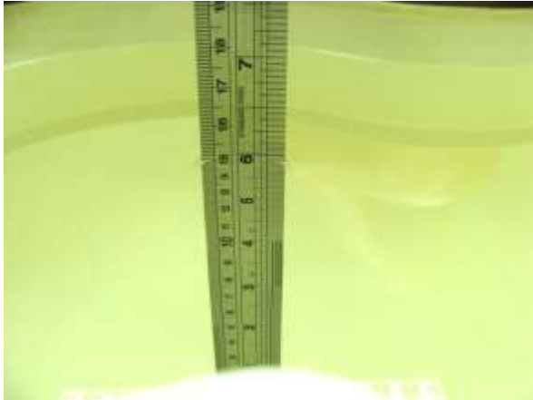
Fig 6.1 Photo of Liquid Height for Head SAR
