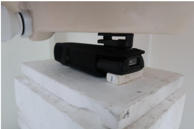
Front with Holster 1, Test Separation 0 mm
