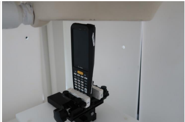
Top Side, Test Separation 10 mm
