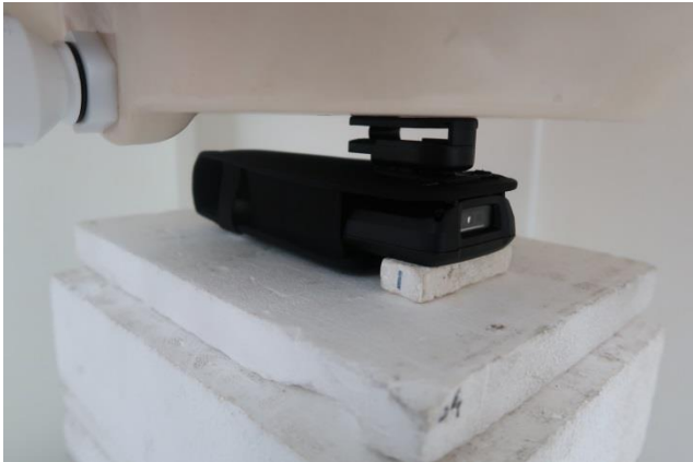
Front with Holster 1, Test Separation 0 mm
