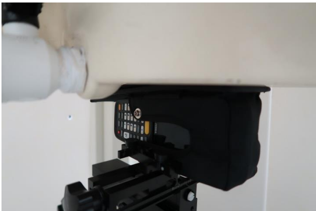
Left Side with Hoster2+Trigger Handle, Test Separation 0 mm
