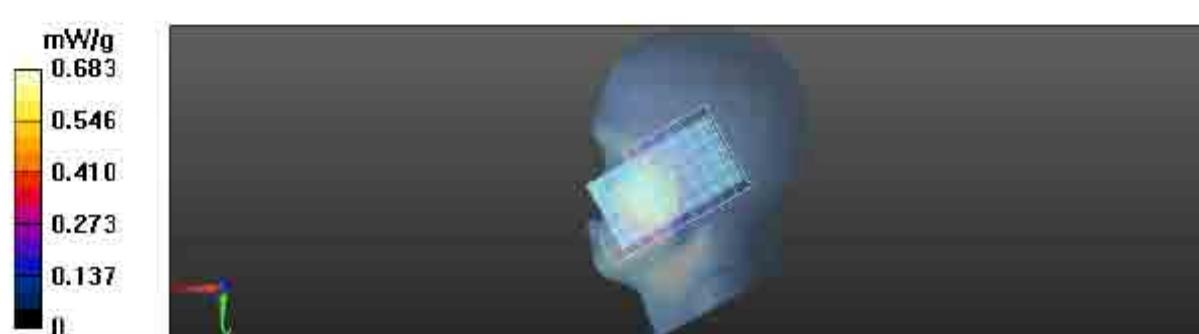
Shortened scan reflect highest SAR producing configuration; approximate run time is 7 minutes.
